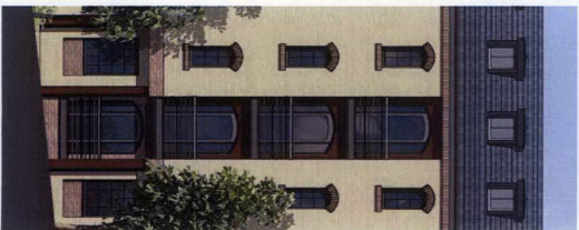
Coloured and brick infill panels with large arched openings
